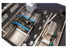
The servo-motor is employed for knife driving to provide high speed and sharp fore-edge trimming. The topbottom transport belt insures smooth booklet transportation and delivery. Trimmings are blown down into the external trim box by air so that no chips are left in the trimming area. Durable casting structure maintains the quality trimming.
