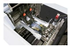
The wire feeding sensor alerts when the wire spool is nearly empty or jamming, and stops the system to eliminate non-stitched booklets. Up to 48 sheets of normal paper (64 gsm / 50lb. offset) can be stitched or up to 24 sheets of normal paper (64 gsm / 50lb. offset) can be stitched and folded. The stitching position and distance are automatically set up for the input size.
