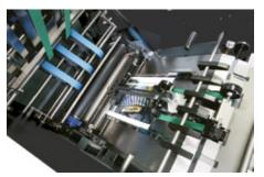
Folding roller and press roller gaps are automatically adjusted according to the booklet thickness. The jog sensor detects jog faults and rejects any errored booklets to the reject tray. Sheets are firmly registered with tail edge and top-bottom guides to provide accurate folds.
